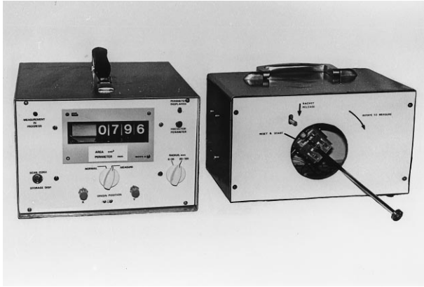
Fig. 21. The first electronic area and perimeter measuring device for ultrasound images (Fleming and Hall 1978). (From BMUS Collection.)
