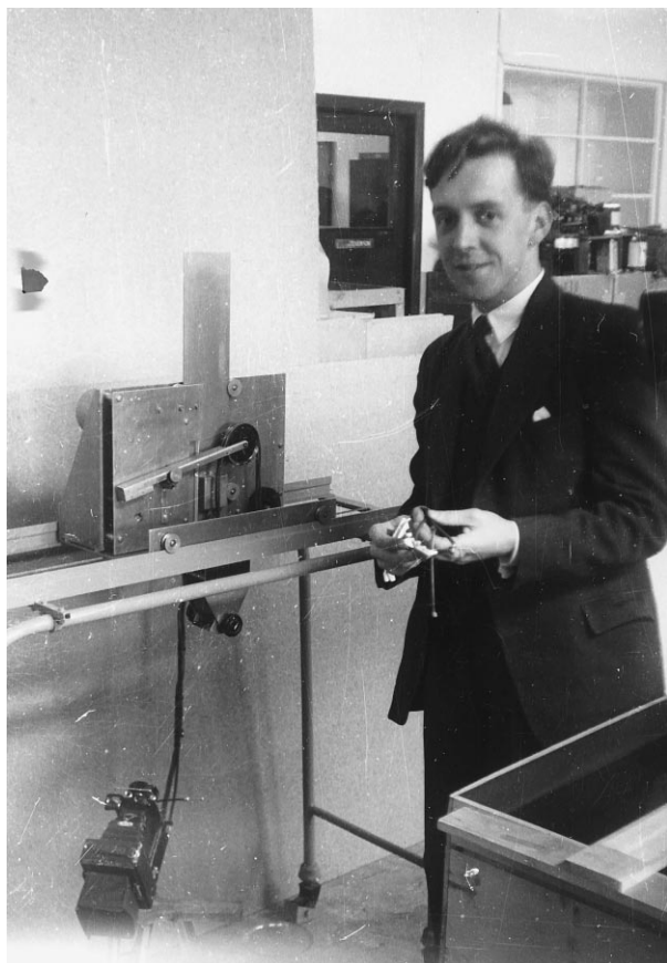
Fig. 3. Tom Brown with the first contact scanner in the development laboratory at Kelvin Hughes Ltd., Glasgow, 1957. This machine commonly is referred to as the "bed table machine," as a hospital bed table was used to support the scanning mechanism. (From BMUS Collection.)
