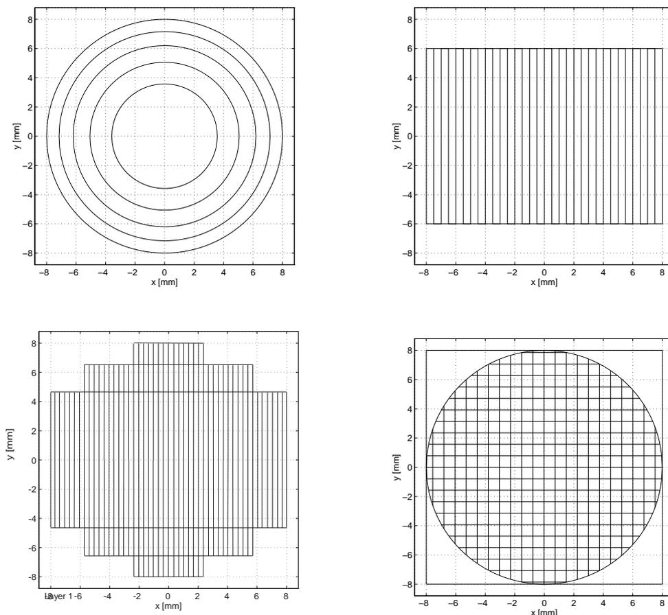
**Fig. 1. Array types: Annular array, rectangular array, 1.5D array, and 2D array**
