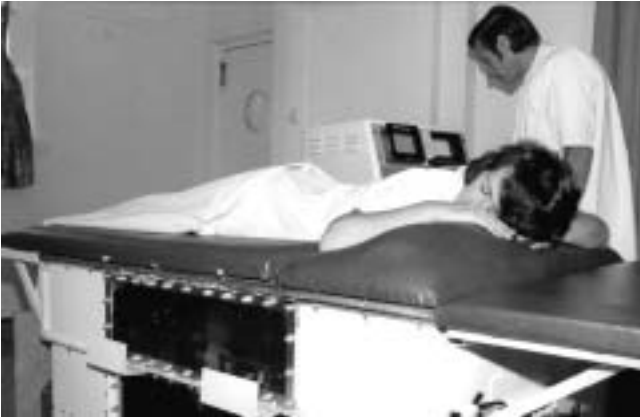
Figure 5 UI Octoson. Eight transducers encased within a water bath, allowing the patient to easily lie on a plastic membrane.
