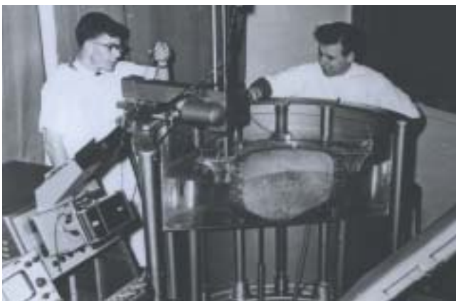
Figure 1a CAL MKI Abdominal echoscope, under construction. Left David Robinson, right George Kossoff
