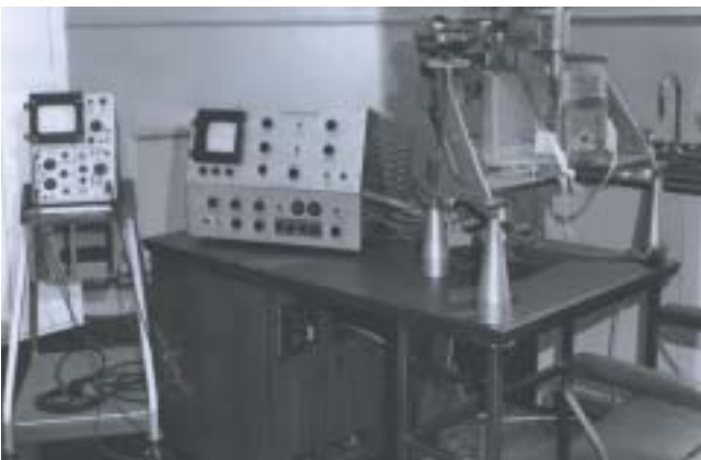
Figure 6 CAL Eye echoscope with patient coupling on the right and recording equipment on the left.
